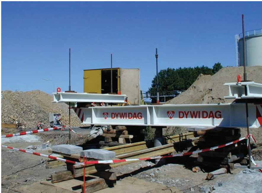
Static pile test
