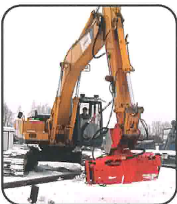
Movax TPH - foundation hammer - "PDA" can be seen on the monitor
