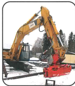
Movax TPH - foundation hammer - "PDA" can be seen on the monitor
